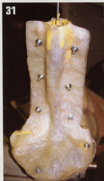
31. The partly-filled epoxy resin mold was turned in a vise so that the knee opening with the second end of the threaded rod showed to the top. Now the rest of the mold was filled with chromium oxide
